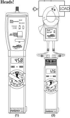
Connect to Fieldpiece accessory heads by simply attaching them to the top of meter (1) or attach remotely through leads (2). For most heads, move dial to mVDC range shown (1). For the AAC clamp (ACH4), move dial to VAC range (2).
