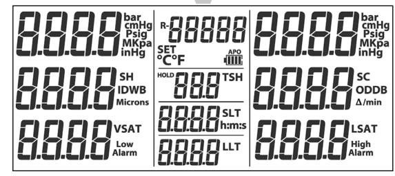
Pressure (bar) bar Pressure (pounds/in<sup>2</sup>) Psig Pressure (kilopascals or N MkPa Negative Pressure (inche inHg Negative Pressure (cm of cmHg Superheat SH SC Subcooling **Target Superheat** TSH SLT Suction Line Temperatur LLT Liquid Line Temperature VSAT Vapor Saturation Temper
